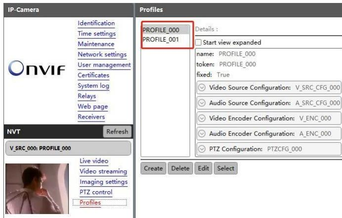
If <video\_source>.width and <video\_source>.height of multiple <profile> tags are not the same, it is considered that they are using different video sources,
